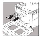
Place the machine in an upright position and remove the three plastic bolts.
